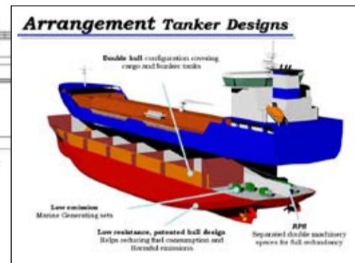
Ecoship 14700 dwt. Chemical & Oil Tanker Ship designs. Twin propeller 6,4 MWe diesel-electric Redundant Propulsion System with SCR exhaust emission control system.
